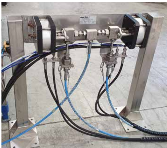
↑ Bi mode valve ass.y: BMC-1A2U-3000-V2x Installed inplace- connected with hoses to gun Device for safety selection of gun 1 / gun 2
