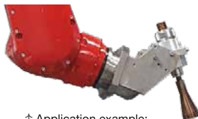
↑ Application example: automatic gun on Robot
