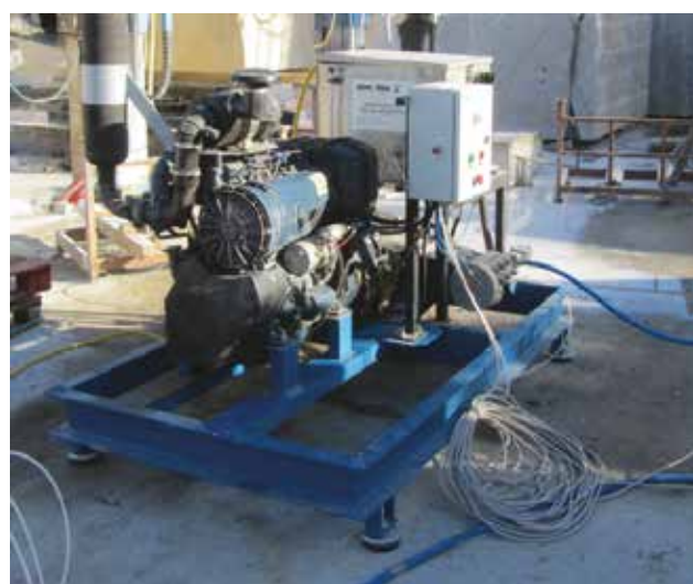
↑ Fully autonomous high-pressure unit powered by a diesel engine.
