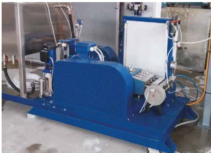
↑ Ultra-high-pressure unit with direct connection to a water-flame module (45 kW). Units available in capacities ranging from 37 to 90 kW.
